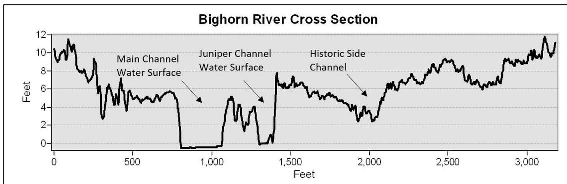
**Figure 8. LiDAR cross section showing multiple current channels (water surface) and historic channels (ground surface) channels. Location of the cross section is shown in Figure 9.**
