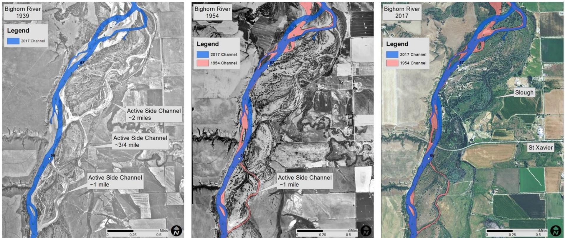
Figure 40. Progressive loss of several miles of side channels near St Xavier between 1939 (left) and 2017 (right)—flow direction is to north.
