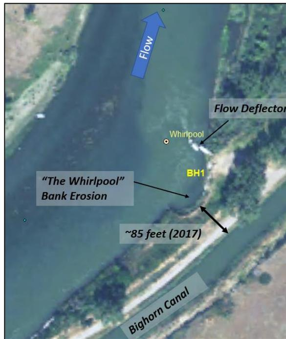
Figure 20. 2017 air photo showing scour upstream of flow deflector; back eddy has eroded the bank towards Bighorn Canal.
