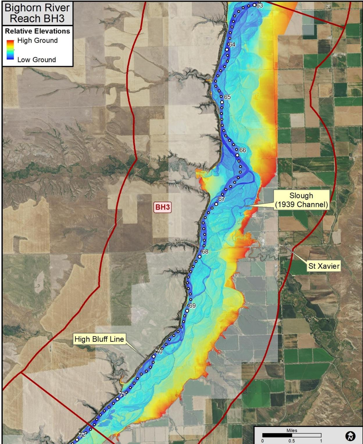
Figure 38. Reach BH3 showing relative elevations and major features.
