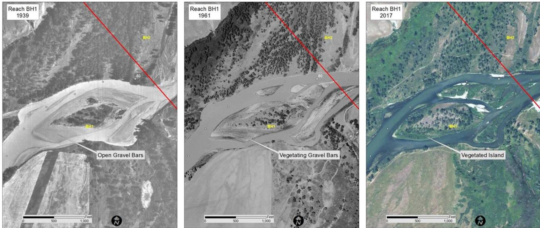
**Figure 21. Comparison of section of BH1 just upstream of Three Mile showing side channel loss and vegetation encroachment since 1939—flow direction is left to right**
