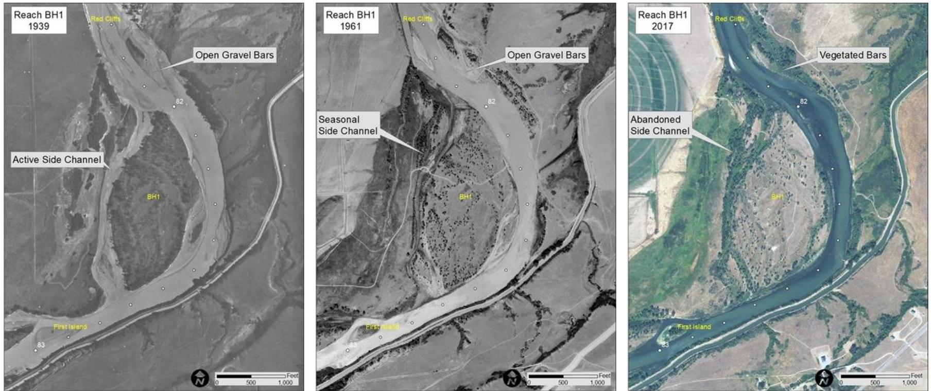
Figure 18. Comparison of section of BH1 upstream of Red Cliffs showing side channel loss and vegetation encroachment since 1939—flow direction is to north.
