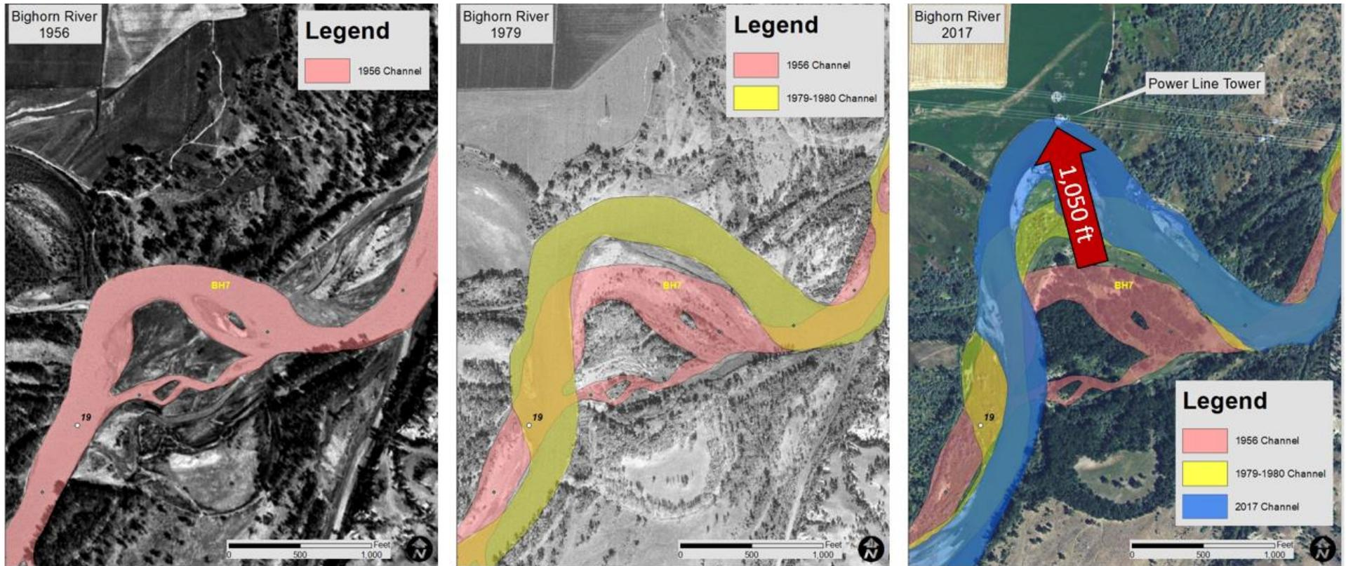
Figure 49. Northward migration of a large meander into a power line tower from 1956 to 2017; bank has moved over a thousand feet into infrastructure/irrigated field. Flow is to northeast.
