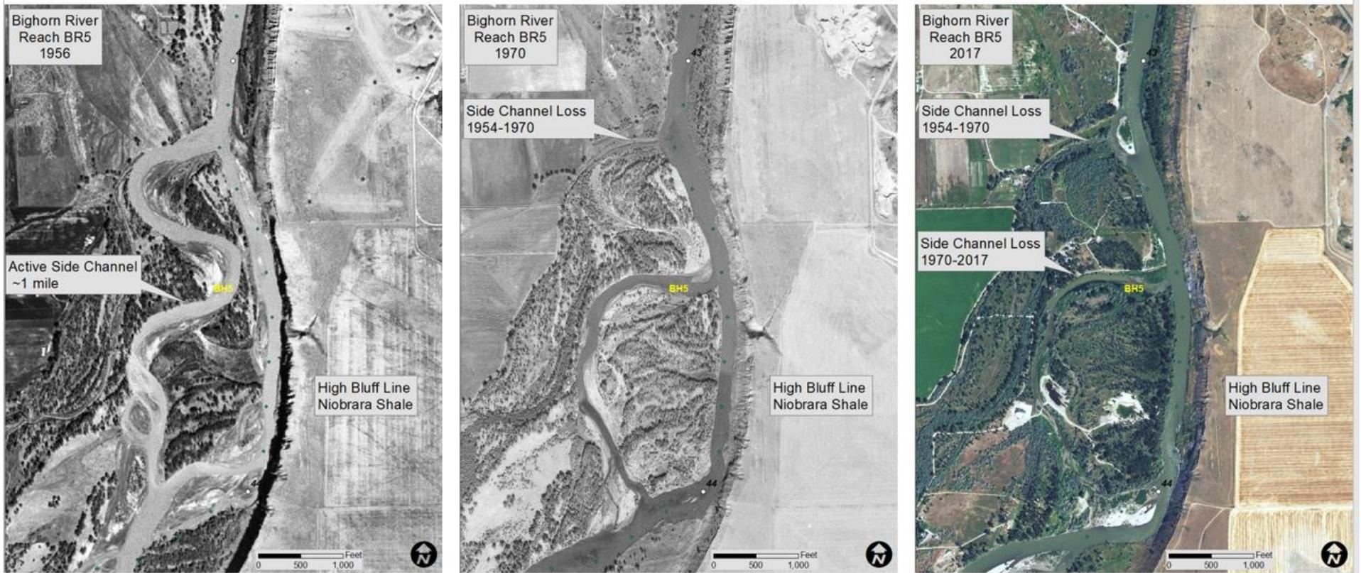
Figure 44. Progressive loss of a ~1 mile long side channel in northern portion of Reach BR5—flow direction is to north.
