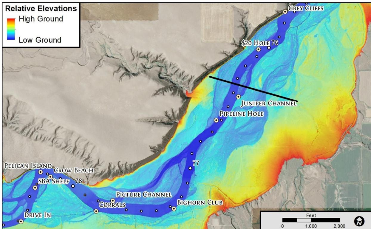
Figure 9. Relative Elevation Modeling (REM) using LiDAR elevation data with cross section location.
