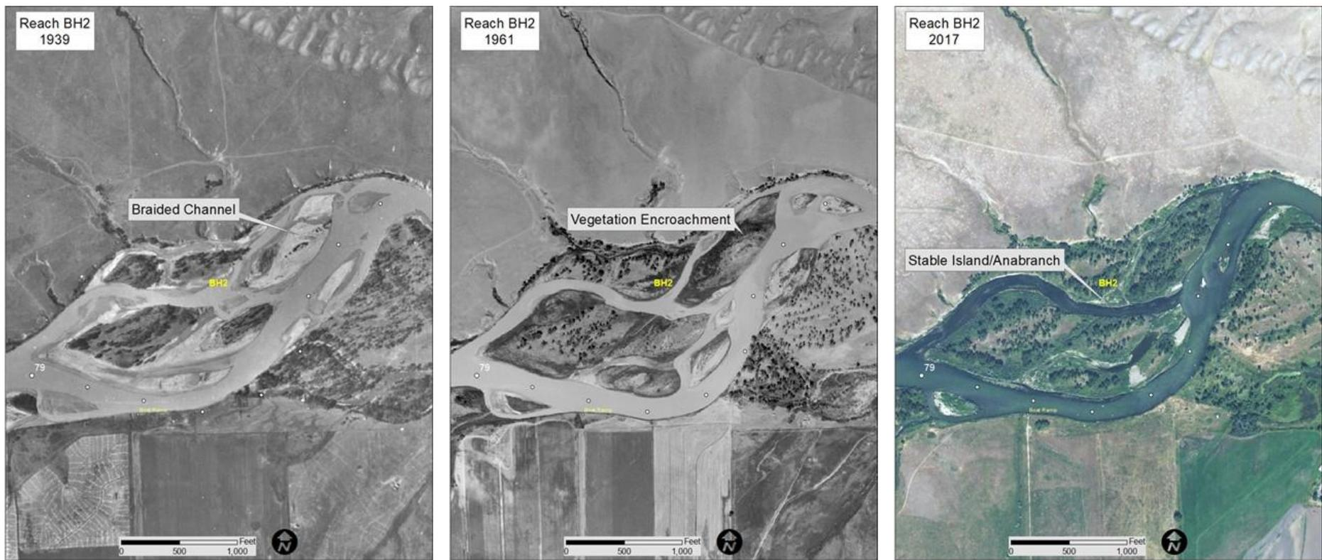
Figure 35. Comparison of section of BH2 at Duck Blind Channel showing channel simplification since 1939—flow direction is left to right.
