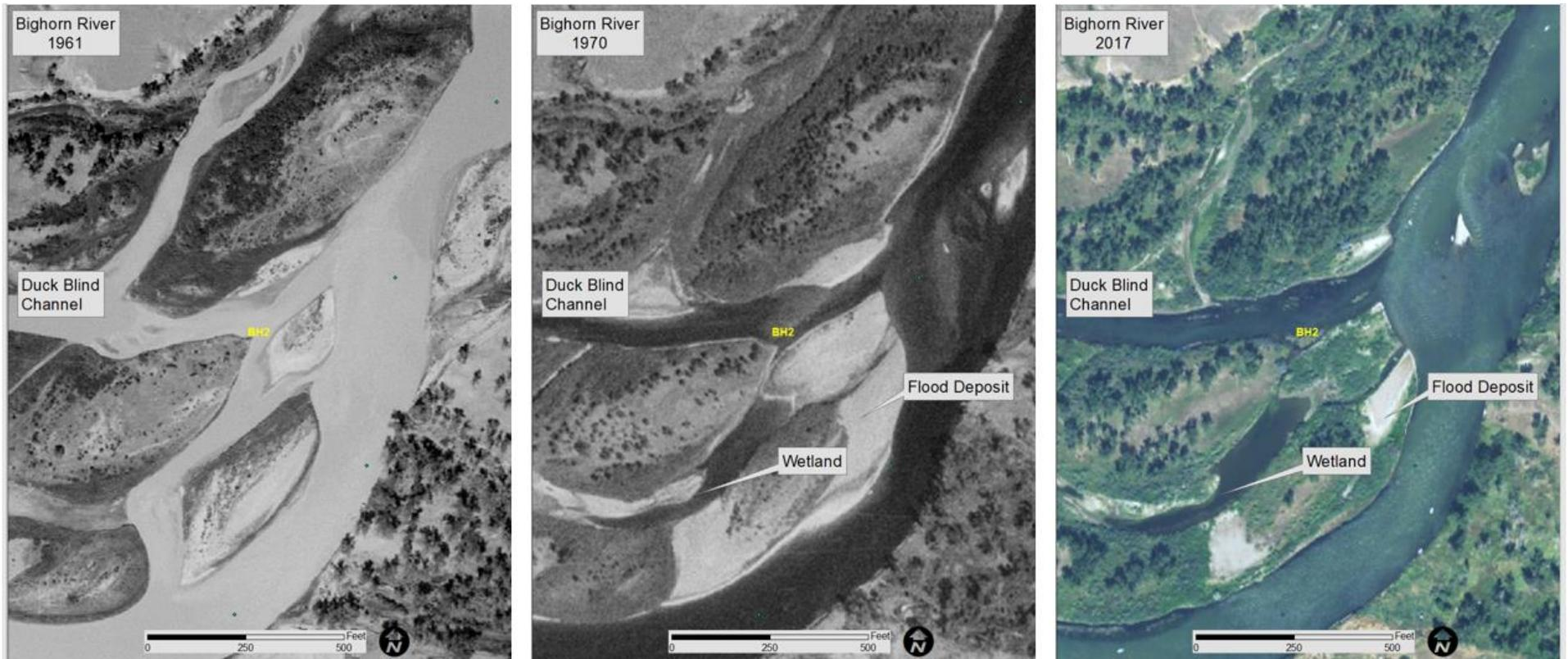
Figure 34. Comparison of section of BH2 at Duck Blind Channel showing flood deposits established between 1961 and 1970—flow direction is to northeast.
