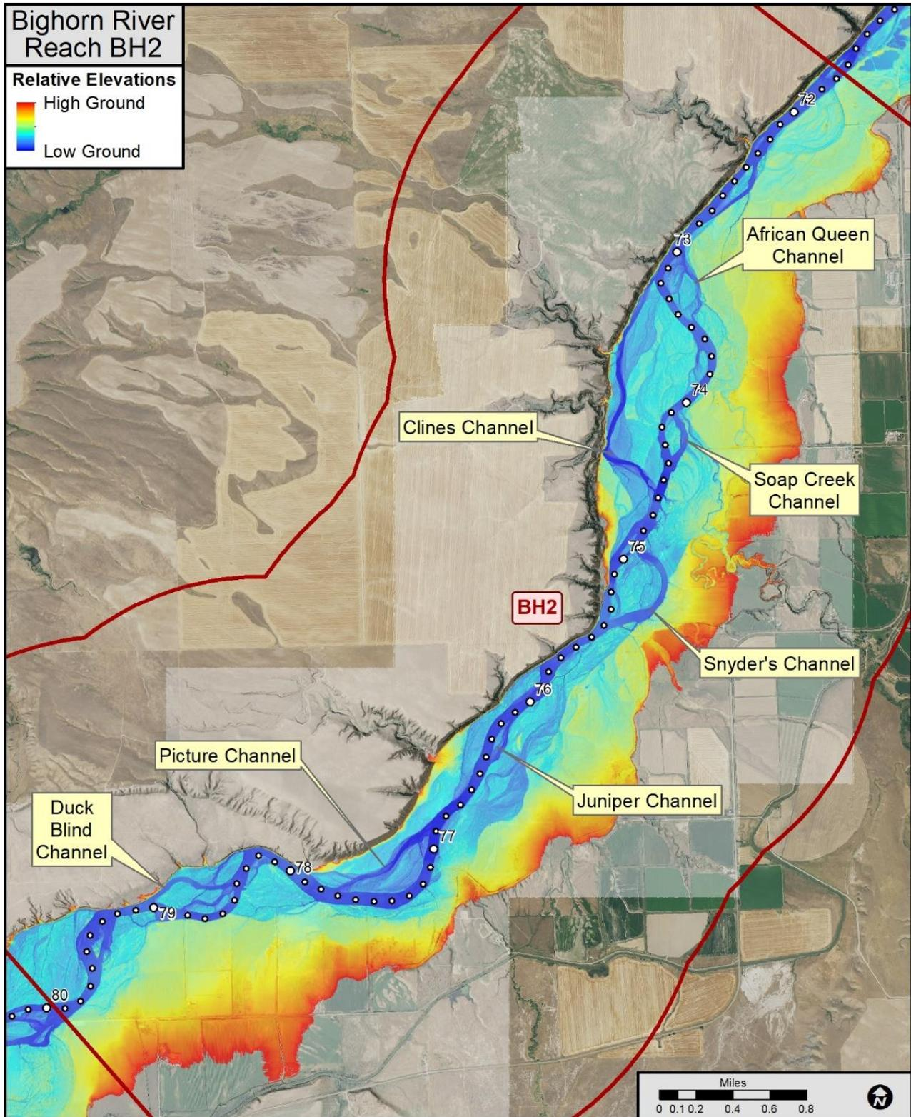
Figure 25. Relative Elevation Model (REM) map showing major side channels in Reach BH2.
